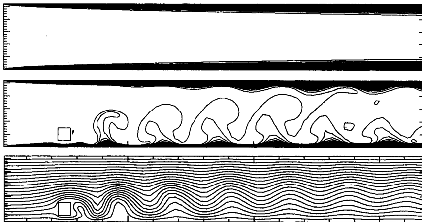
Figure 11. Instantaneous temperature contours and streamlines for the flow past a square cylinder in a channel with heated sliding walls and \alpha=0^\circ , h/H=0.192 ( g/d=0.5 ), d/H=0.192 , Re=500 . Temperature contours without the cylinder (top); temperature contours with the cylinder (middle); streamlines corresponding to middle plot (bottom)
